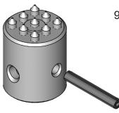
9-POINT TUNGSTEN CARBIDE BIT WITH H.D. COILED SPRING PIN PART # 18820 5 REQUIRED
